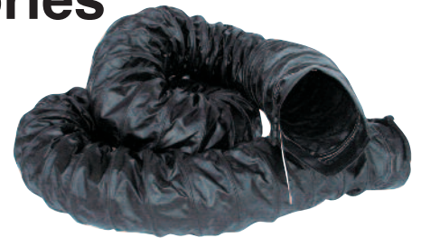
Conductive Ducting With Ground Wires Attached to Each End of Wire Helix
