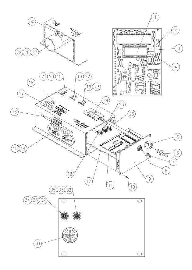
**NOTE:** Model CO-91IS has the indicator lights and audible alarm mounted on bottom of housing and model CO-91ISLA has the indicator lights mounted on top of housing with the audible alarm being mounted on the left endplate.
