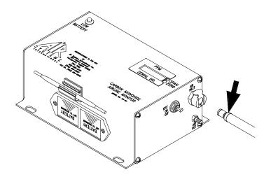
**STEP 2)** Connect the air sample hose to the monitor.
