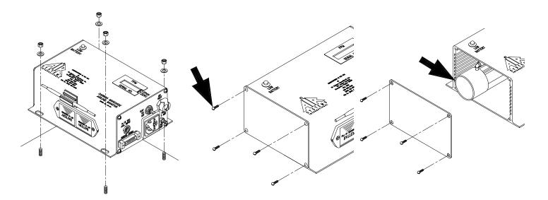
Step 1) Disconnect all external connections. Remove CO monitor from the unit.
