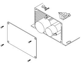
STEP 1) Disconnect all external connections and remove CO/O2 monitor from the unit.
