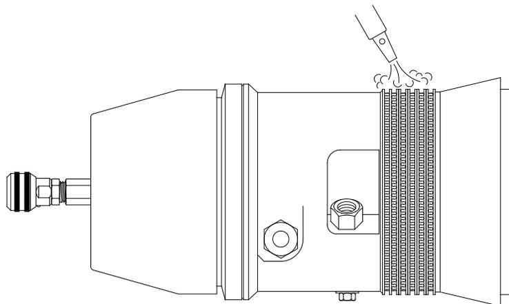
**Blow dust off of oil cooler periodically to prevent over-heating.**
