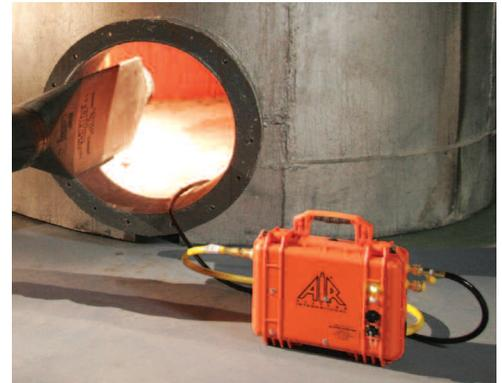
The Breather Box® portable air filtration system is designed to filter incoming air from a compressor to provide airline respirator users Grade-D quality air while monitoring for CO and/or O<sub>2</sub>.
