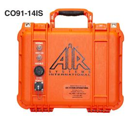
A portable airline monitor connects easily to a breathing air filtration source or ambient air pumps and monitors the air for CO or  $\mathrm{CO/O_2}$ , depending on the model. An audible alarm (95 dBA) and light will activate when the CO level exceeds 10 ppm (5 ppm Canadian). Used in the closed and upright position, an external alarm and lights signal the user if there are dangerous CO or  $\mathrm{CO/O_2}$  levels.
