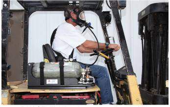
PAK-SFL™ & bracket mounted on forklift
