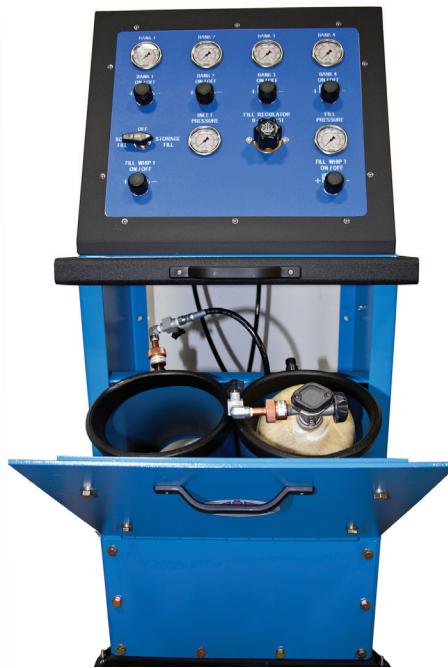
2 Position Fill Station open
