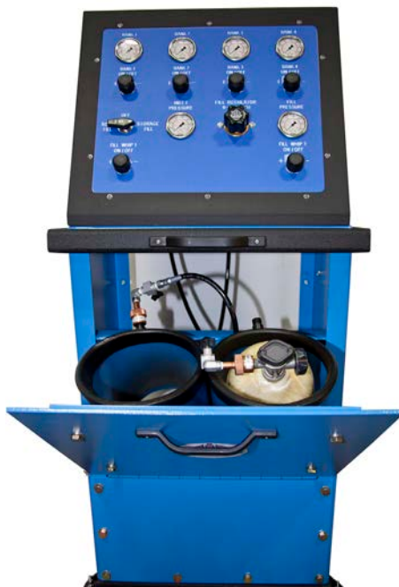
2 Position Fill Station Open
