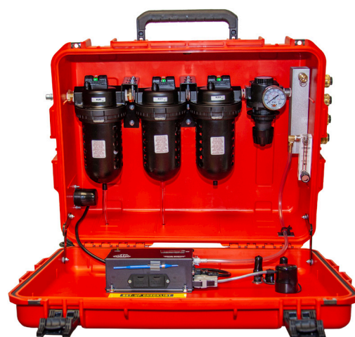
BB100-CO Series 100 cfm Breather Box® 123 cfm flow capacity 4 to 8 couplings available
