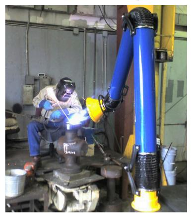
The steel Fume-Air<sup>™</sup> 750 HEPA filtered fume extractor provides 750 cfm flow through a 13" hood and is ideal for welding and soldering applications where large flow volume is required. With 270 degree movement and 10 foot arm length, it is easy to position the hood next to the welding work.
